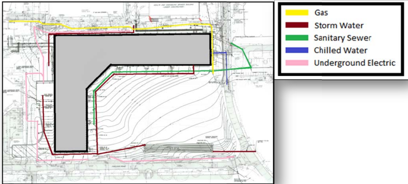
Figure 10: Final Site Utilities Plan
